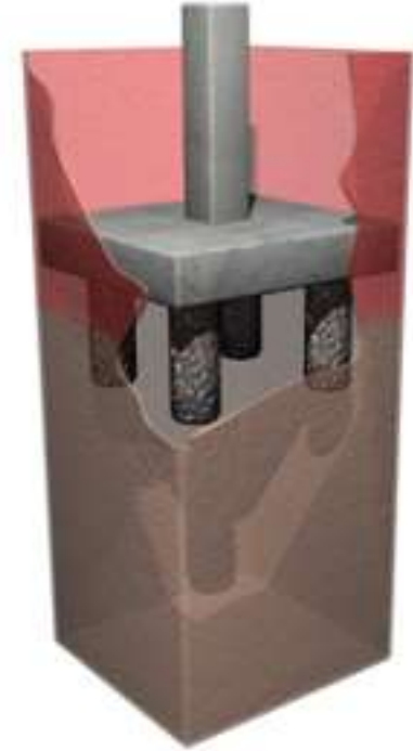
Figure 2 (vibro stone columns & raft)
